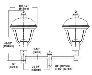
Post Top with BK MPT BO (x2) Mounts to 4" or 5" Dia. D180 Bolt-on Pole (select 3" reduced drilling pattern)
