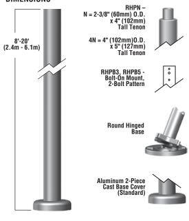
**POLE SHAFT** - The pole shaft is extruded from seamless alloy aluminum. Tenon N option is 2-3/8" O.D. x 4" tall. Tenon 4N option is 4" O.D. x 5" tall. Aluminum round poles are 4" and 5" in diameter.
