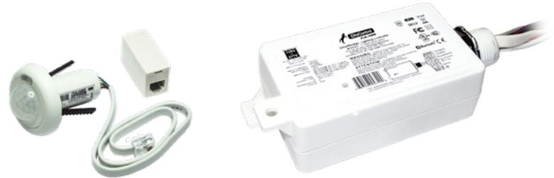
The AirLink Blue Circuit Controller and Ceiling Motion/Daylight Harvesting Sensor provides wireless lighting control based on motion and available ambient daylight. Multiple fixtures can be grouped to be controlled by a single sensor. Controls 0-10 VDC LED drivers and is rated for indoor installations. Utilizes a Bluetooth Low Energy (BLE) mesh network. Dim levels and schedules can be set through LSI AirLink Blue iOS app.
