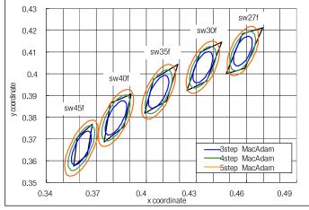
Deco Lighting uses only the finest LEDs made by Nichia, the world's largest LED manufacturer. The Nichia LED is considered the Rolls Royce of LEDs. Featuring a 3-step MacAdam ellipse, the tightest binning in the industry, Nichia LEDs are held to a higher standard than minimum industry requirement and don't color-shift like fixtures utilizing lower quality LEDs.
