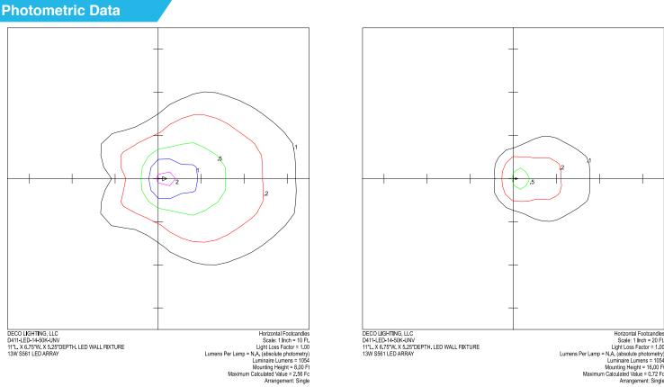
Horizontial Footcandies Scale: 1 Inch = 20 F. Lüght Loss Factor = 1.00 Lumens Per Lamp = N.A. (absolute photometry) Luminaire Lumens = 1054 Mounting Height = 16.00 Ft Maximum Calculated Value = 0.72 Fc Arrangement: Single
