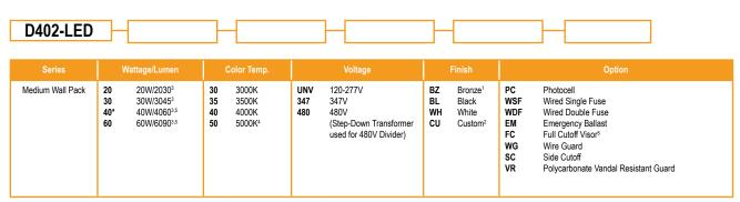
\*Select-A-Watt model, factory set at listed wattage when shipped. Please contact factory for information on selectable wattages for this fixture.
