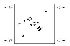
3) Mount back plate to surface using the provided slots. Use temporary hanging cable and hook for ease of installation.
